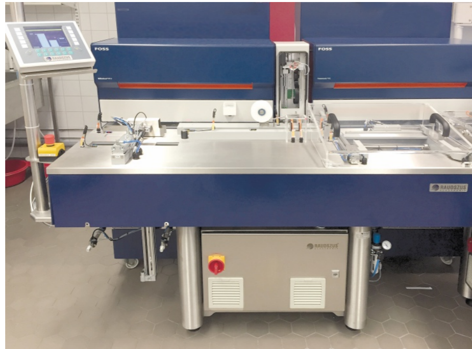
Basic Unit - to handle the samples in front of an Analysing Unit
