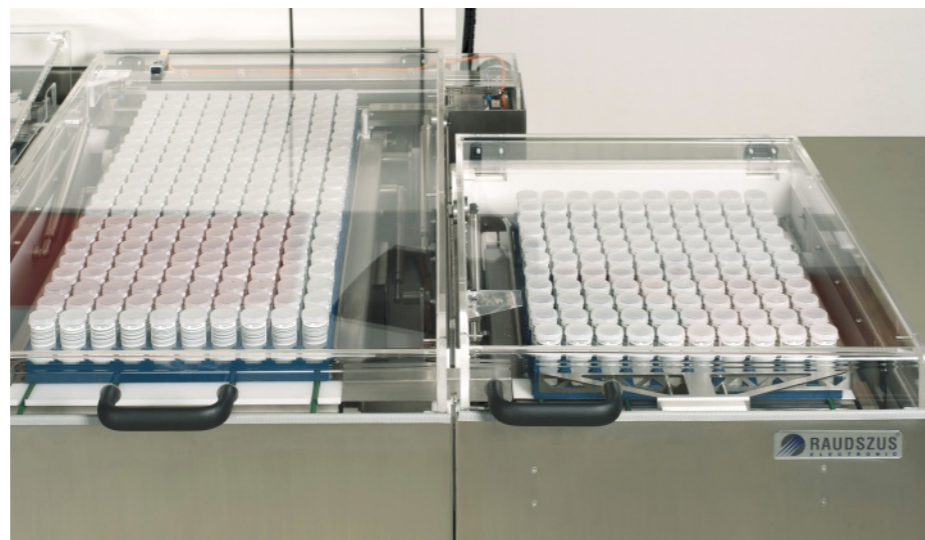
Warming Area - to warm up the samples by warm air
